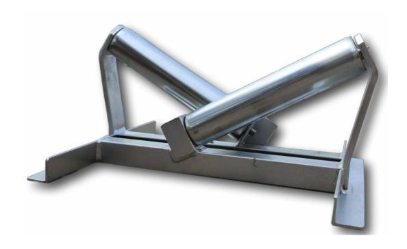
The V style cable roller leads the cable from the drum into the trench, the design is such that cable is centralised prior to it being fed into the trench. This roller also doubles up as a heavy duty straight line roller or pipe roller and can be positioned in the trench itself. Any width or capacity of V roller can be made on request
